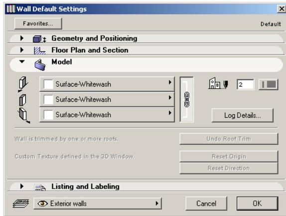
The most important control of this panel concerns the surfaces of the wall's two sides and all four edges. Clicking the chain icon will assign the last material chosen to all surfaces. Deselecting the chain icon will restore the materials that you originally set for each separate wall surface.
