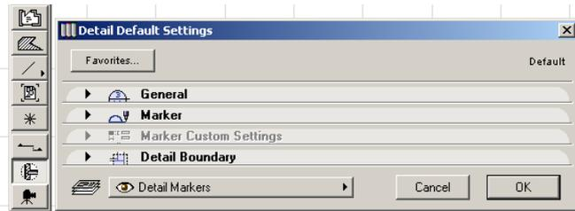
The **General** panel contains the identification of the Detail Marker and its placement angle.
