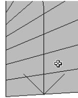
Press and hold the mouse button while moving it along the stair. Some treads turn white as you make the winder section shorter at the end. Release the mouse button, and StairMaker will show the new outline of the stair. Make sure that you define a winder section without overly skewed treads.
