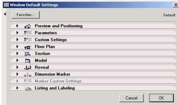
There are ten panels in the Window and Door Settings dialog box: Preview and Positioning, Parameters, Custom Settings, Floor Plan, Section, Model, Reveal, Dimension Marker, Marker Custom Settings and Listing and Labeling.
