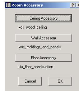
When pressing **OK**, Interior Wizard places the Accessory Objects on the surface of the 3D Zones. If the given room's Zone is changed or updated, use the **Update Room Accessories** command from the **Interior Wizard** menu to update the placed Accessory Objects.
