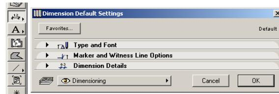
The Dimension tool's setting dialog box includes three panels: Type and Font, Marker and Witness Line Options and Dimension Details. Note that some of the other dimensioning tools have single-panel dialog boxes.
